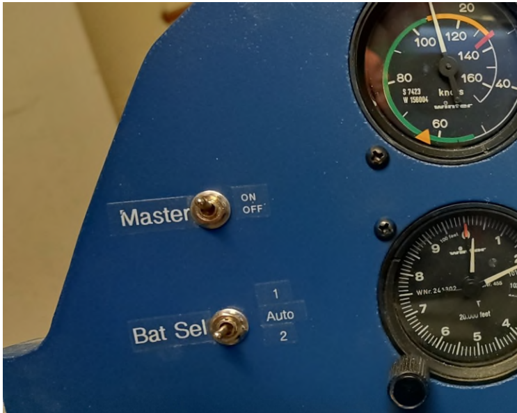
Typical GBMS system installation. NOTE the AUTO position
