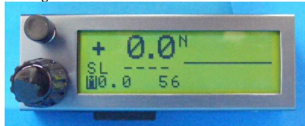
In both climb and cruise the dotted line is the current 20 second average value, TE variometer in climb, Netto in cruise.
