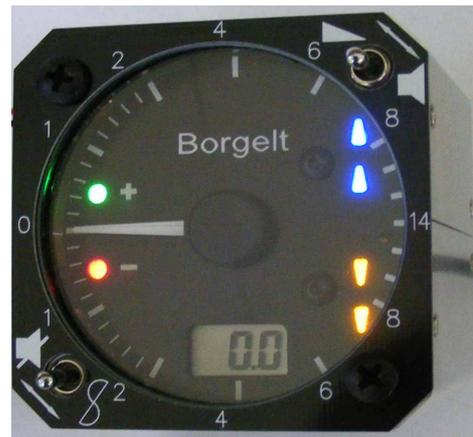
**1.1 Climb Mode** (Mode or cruise/climb switch closed – Note mode switch sense can be inverted in customer software setup for gliders with the switch installed in reverse)
