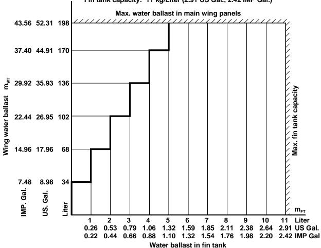
Always full Liters are to be filled. Where value jumps, either Note: the higher or the lower amount of ballast may be used
