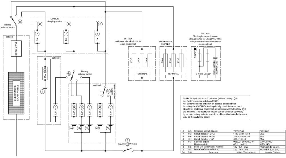
Solar panels to be wired at the main power supply only by regulator with  $V_{max} = 13.8V$
