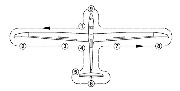
When walking around the "Duo Discus", check all surfaces for paint cracks, dents and unevenness.
