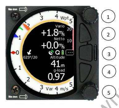
1 - Rotary switch with push button Enter and operate only in the volume menu
