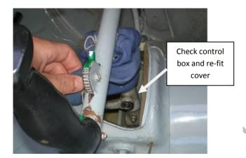
Figure 3 inspection of brakes and control box
